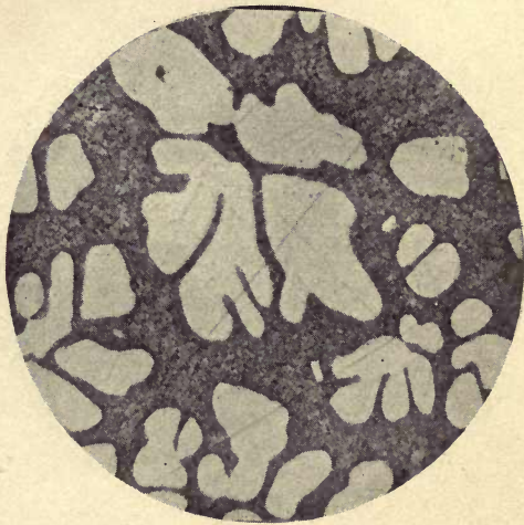
Fig. 33a. \times 700 Alloy 54. Cu 58.0 Sn 8.0 Zn 34.0 Slowly cooled in furnace. \gamma -Segregate + app. \beta .
